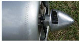
The propeller blades broke off at the hub in flight while the motor kept running – not much thrust though! This is another reminder of why we mustn't stand in line with spinning props.
