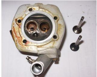
Once all the carbon was removed it was time for reassembly. The tricky part is fitting the tiny valve retaining collets. Extreme care must be taken because if you slip off the retaining washer while depressing the spring they can be flung in all directions and lost. I did this part on the kitchen table because they would be easier to find inside rather than on the garage floor.
