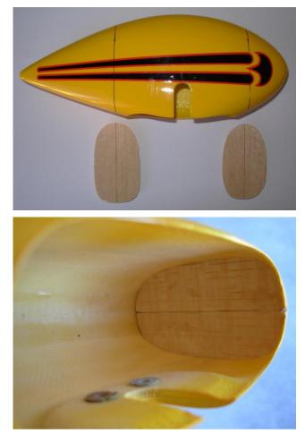
The formers were then epoxied in place along with the extra outer side plate (not shown here) to produce a very strong and hopefully serviceable wheel spat.
