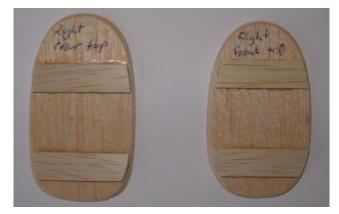
The drawing was then printed and the four (two the same) formers cut out from the sheet as a rectangle and stuck to hard 1/8" balsa using 3M spray adhesive then cut out on scroll saw. A chamfer was then sanded on one edge and with very little adjustment they fitted the required location. As you can appreciated with the
