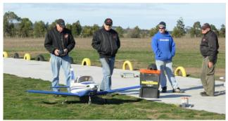
Glenn is taxiing the Airtourer out to the runway for the test flight with a nervous Mike looking on. The Airtourer is built from a Scale Aviation Australia kit, is powered by a DA50 petrol motor and has JR PCM10X radio with 2.4GHz module. Murri Anstis (right) was the HM inspector.
