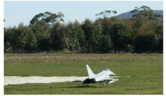
The Eurofighter is on the verge of lift off. You can see the upward deflection of the elevons to lift the nose.
