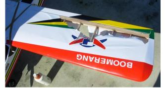
The covering tore away on the upper and lower surfaces of the left wing during the first flight. Very unusual!!!
