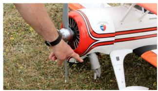
News flash!!! Roger had two dead stick landings with his Super Stearman. The first was attributable to a lean mixture whilst the second the muffler came loose on the OS200FS and dropped down severing the pressure line. A1 is kindly pointing this fact out to Glenn with the camera. Muffler was retightened and the pressure line reattached, followed by a couple of uneventful flights.
