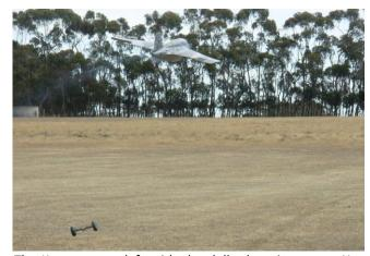
The Komet gets aloft with the dolly dropping away. You can see the elevon control deflection in the photo. Lots of left being applied here. It's all happenings on take-off that's for sure. The trees in the background are on the northern boundary and are a long way from the flight line. The worst thing is when landing from the north your model tends to get camouflaged making it difficult to see under some light conditions.
