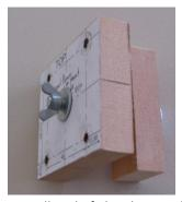
The drill template was then clamped to the firewall through the fuel tank neck locating hole using a coach bolt through a block inside the fuselage and secured with a wing nut. The alignment on the firewall was critical to ensure that the correct thrust line was maintained and the
