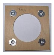
Because the holes in the firewall were plugged and drilled I decided to cut out a supplementary plywood plate (left) to hold the blind nuts. This was then epoxied to the inside of the firewall using the 10-32 bolts to clamp it in place while the epoxy hardened. It also meant
