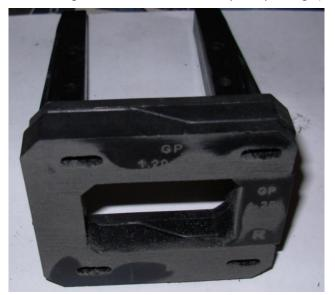
Mounting surface has been faced off carefully on bench belt sander. It is surprising how uneven they are! 100% contact isn't necessary but it needs to be around the mounting holes.
