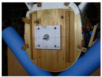
The engine mount drill plate is bolted to the firewall through the fuel tank neck locating hole in precisely the correct location using registration marks. The four holes are then drilled through the firewall using a hand held drill. The drill block ensures perpendicular holes.
