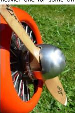
engine and plane would perform better with an APC 18x8 or 18x10 prop instead of the lighter 18x8 Zinger wood prop.
