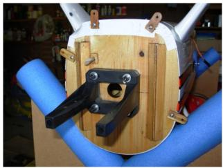
The new 180 size mount bolted on to the firewall replacing the lighter 120 size mount.
