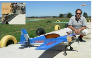
Nick's Edge 540T in the pits on Sunday 30<sup>th</sup> January for an engine run up. Note the muffler (see inset photo) Nick has fabricated this to keep the muffler within the cowl and model needed the weight in the nose.
