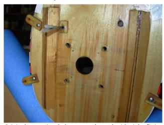
Original mounting holes were plugged with tight fitting dowel and redrilled using a drill block clamped to the bulkhead through the fuel tank neck locating hole.
