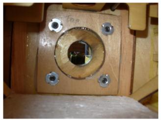
Inside shot of the firewall showing the supplementary plywood plate and blind nuts epoxied in place. Fuselage is upside down here — the white polystyrene foam in the bottom of the photo contains the Batteries & Receiver. It was cut to mould into the contours of the fuselage top. All originally done to get the CofG correct with minimal ballast.
