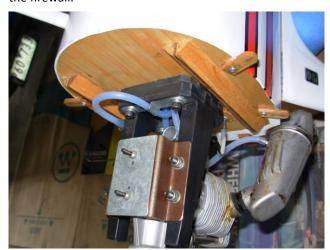
OS200 FS refitted to the new heavier mount with new fuel line retaining clamp. The ballast mount has always been fitted but no longer has any lead.
