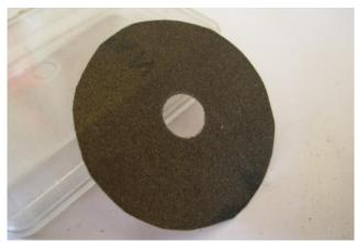
Friction disc made from 220 grit carborundum paper. The 40mm diameter disc was needed to prevent prop slipping on a spacer washer.
