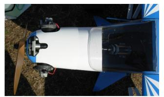
Note the onboard electric starter mechanism.
