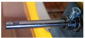
All you need is a small flat for the screw to seat on and don't run the flat all the way to the end of the axle which might still allow the collet to slide off.
