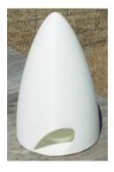
Peter has been doing some experimenting with 3D printing of aero modelling parts. Last Sunday (23<sup>rd</sup> February) he brought out a spinner that was 'printed' using a machine that costs around \$2500. The spinner has a 100mm diameter and took 4 hours to print, however it is non-structural and could not be used. The surface wasn't perfectly smooth but with a
