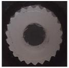
Sanwa servo output shaft is 5.95mm diameter and has 23 teeth like JR.
