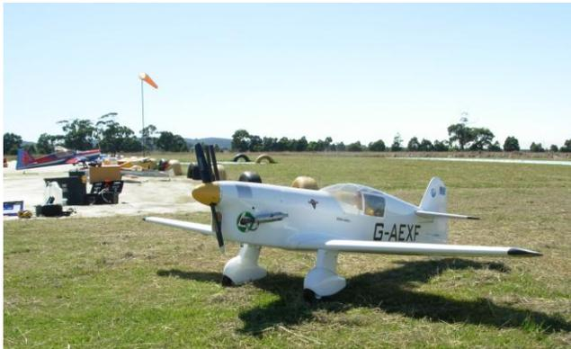
*Glenn's latest model – a 74" span Mew Gull ARF powered by an early model OS120FS.*
