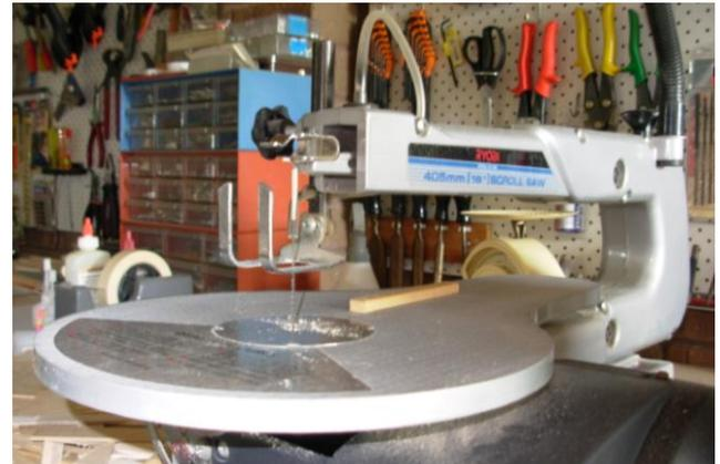
*Masking tape on the upper teeth of your scroll saw blades readily identifies the top side of the blade and helps to prevent cut thumbs while fitting blades. Note aluminium table insert.*
