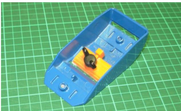
*I've always found adjusting the blade in razor plane a hit & miss affair. Sitting plane on cutting mat while lightly pressing blade holder and thus blade onto cutting mat then tightening seems to produce a reasonable cutting depth.*
