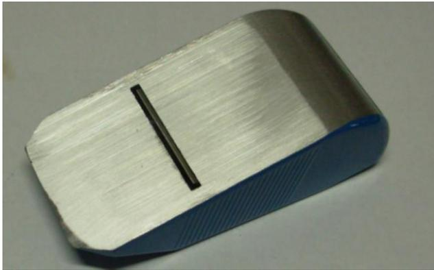
*Make sure the base of your razor plane is flat – mine definitely wasn't making cuts unpredictable.*
