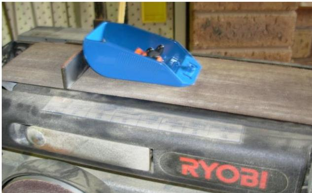
*Squaring off the base of razor plane on belt sander – this made a remarkable difference to ease of use and effectiveness. Best to take the blade out first!!!*
