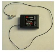
JR RS10DS 10 Channel Receiver 36MHz PLL Synthesized \$30. (Note: Aerial wire will need reinstating to the correct length.)
