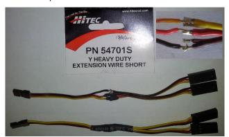
Inset, you can see the open joint on one of the black leads. With the heat shrink tubing everything looks peachy but beneath one never knows how good the soldered joint is.
