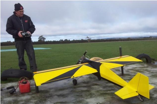
Max with his Hots powered by a 3MM 53cc petrol engine doing engine run up tests. Looks like it should have plenty of power.
