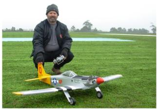
David Filmer can be seen here with his new Hanger 9 PTS (Progressive Trainer System) P51 Mustang Trainer, powered by an Evolution 40 two stroke motor. Model comes with trainer aids: Clear aerofoil sections taped to the leading edge of the outer wing panels, speed brake system on the fixed L/G and two position flaps that can be rigged up to a servo.
