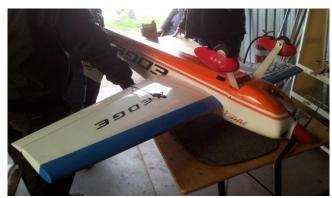
Photo taken last month after the servo shaft sheared. The Edge is about 72" span and powered by an OS120 2 stroke.
