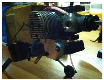
The new GMS 120; showing the new aluminium adapter and the old steel muffler.
