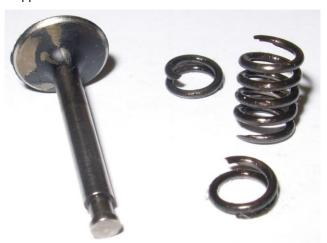
OS91 FS-SII Inlet valve and broken spring. For the record the head is Ø11.2mm, stem is Ø 3mm and 26.4mm long.
