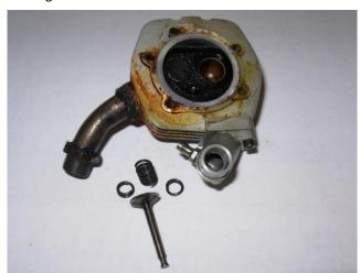
Exhaust valve has also been removed and the carbon deposits cleaned off. I found that an old X-acto blade was an effective tool to scrape the carbon off the valve stem, head and around the seat without fear of scratching.
