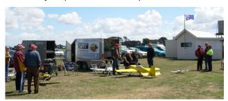
Ken Mollison's big yellow Extra powered by a DLE111. Flew once but suffers from chronic elevator flutter when full power applied. It appears elevator requires static balancing by adding mass to the balance horn.
