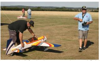
Greg Lepp's ill fated Yak 54. During the second flight (might have been on landing approach going by the scores) it lost radio control and crashed. Apparently the plug lead braiding wore through where it was rubbing on the cowl. The braiding is to shield against radio interference whether 36MHz or 2.4GHz. Rotten luck Greg! Photo was taken while getting ready for first flight. Noel W's Robin less right u/c leg is still on runway in the background.
