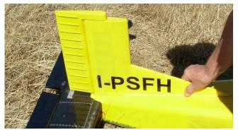
The fin had broken away from the fuselage – one would assume that the fin spars key down into the fuselage.
