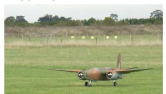
Mike Farnan's WWII Boston powered by two OS Sirius 50cc 5 Cylinder four stroke radial engines. Model is very impressive on the ground and in the air. (Around 3m span)
