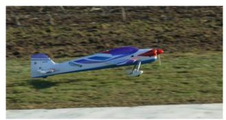
Just managed to snap this shot of Grant's pattern model as it took off. The model is a World Models Groovy 50 3A and from what I could tell flies very well. It has a wing span of 53.5" and is powered by an OS46AX.
