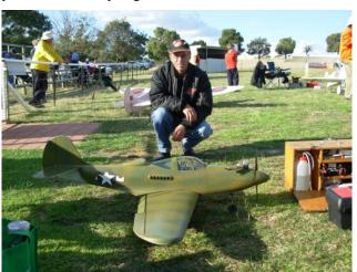
Roger and his old Top Flite P39 Airacobra – originally powered by a Webra 61 2 stroke in 1976 with Kraft Series 75 radio gear. Now has a Magnum 91FS, JR radio gear, but still uses the original Kraft Multicon retracts with separate 650mAh AAA NiMh battery pack.
