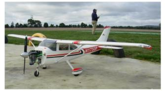
Wayne Goodwin's CM Pro Cessna 182 with Robart sprung nose wheel and OS155FS alpha power. The nose leg is cantered forward about 15° like the full size – I did the same with my TopFlite Cessna 182. I don't think we will see the cowl fitted until Wayne settles on the engine.
