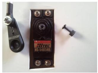
The Karbonite output shaft has sheared under excessive torque load. The ailerons were just too large for this type of servo.
