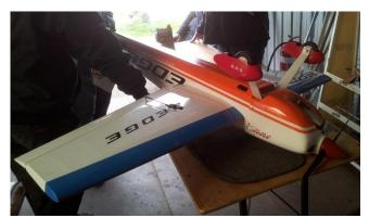
The Edge is about 72" span and powered by an OS120 2 stroke. The ailerons are large on these aerobatic models and therefore impose high load on the servo.
