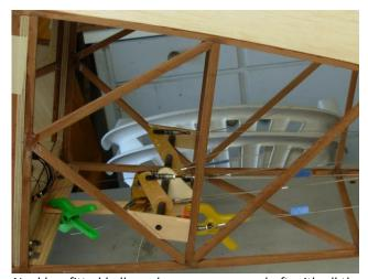
Noel has fitted bell cranks on a common shaft with all the pull/pull cables connected. Pushrods are then connected between the bell cranks and servos mounted in the forward compartment. Cable is plastic coated fishing trace and Noel has tested all cable connection techniques with a 10kg pull test.
