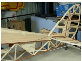
Cables to elevators and rudder exit the side of the fuselage. The elevator cable running over the top of the horizontal stabilizer runs through a felt lubricated guide as per the full size.
