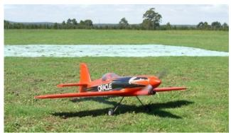
The Turbo Raven is all composite construction. I would say fairly heavy for its size and wing area.
