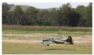
Almost there! By the time it had landed and rolled to a stop, only one motor was running. The problem is the exhaust outlets are fabricated pipes and have no expansion chamber and hence muffler pressure for the fuel tanks. Some modifications will need to be carried out to ensure reliable engines. The model obviously flies very well and all importantly, when it loses motors.
