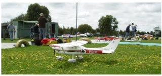
oug Wallis had an unfortunate accident with a Boomerang 60 a few weeks ago. He has since replaced it with the new one pictured below. Doug has fitted a nose leg with a sprung trailing link to improve ground handling and realism.
