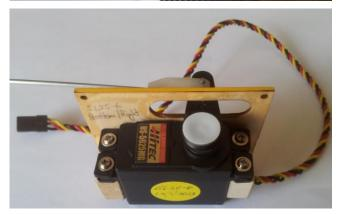
The alternatives are thread locker or a dob of silicone on the screw head and arm, but these are messy to use and can be difficult to undo.
