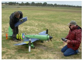
Wayne is now preparing the Westland Wyvern for a flight assisted by John Coughlan. Note the new four bladed propeller for extra ground clearance.
