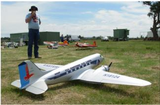
A couple of shots of Wayne's DC3 built from a Top Flyte kit. It is powered by two electric motors, replacing the original 52 four strokes which would not run reliably due to the inherent fuel supply set up.
