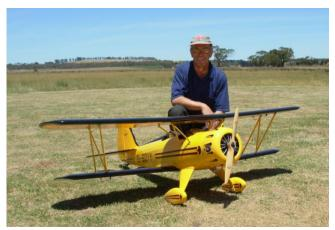
Your editor with his new Great Planes WACO YMF-5 powered by an OS155 Alpha four stroke engine, side mounted with exhaust exiting underneath. The engine is fully enclosed except for the rocker cover which just protrudes through the cowl. I was worried about cooling so fitted ducting plates around the engine to force all the airflow past the cylinder. They are mounted on the removable reinforced dummy engine.
