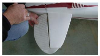
And then we discovered loose elevator hinges – it was time to put the Cessna in the trailer.
