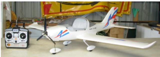
TL 2000 foam electric model complete with geared brushed motor, 4 channel SAPAC radio gear on 36.050MHz. 1150mm wingspan.
