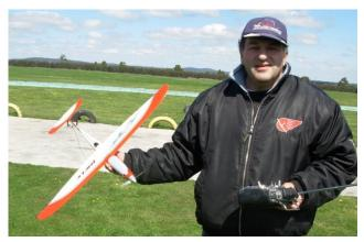
The Rifle is built by Great Planes from fibreglass with a few strands of carbon fibre in the bottom of the wing for extra strength. Aileron-elevator, hand launch and belly landing; it's a slippery little sucker with nothing hanging out. At 31" span and 18oz (785mm, 510g) it is a small, pretty little plane designed to give you a taste for speed, and send you to the optometrist for a new set of glasses.
