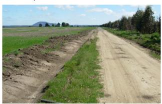
This photo was taken on Sunday 25<sup>th</sup> September. Only a couple of weeks ago the track was under water. The drainage channel, the crushed rock and the recent dry weather has saved our scalps!!!
