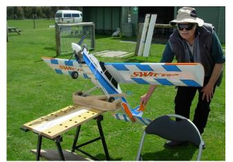
With the arm swung out of the way the nose of the model can be raised while the main wheels are securely restrained in the cradle.
