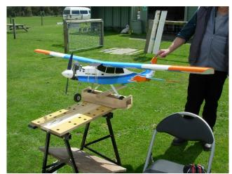
The rear pivoting arm supports the rear fuselage and can be swung out of the way.
