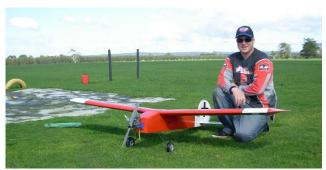
Mat with his latest Graham Waterhouse built Ugly Stik. Model is powered by an NGH 17cc petrol engine and has a wingspan of 2170mm.
