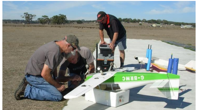
Checking the fuel system to see why the Magnum 91FS would not keep running.
