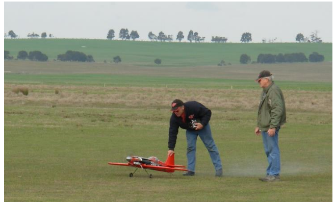
The moment of truth – the first take-off attempt didn't go so well when it swung to the left and broke a blade off the prop.
