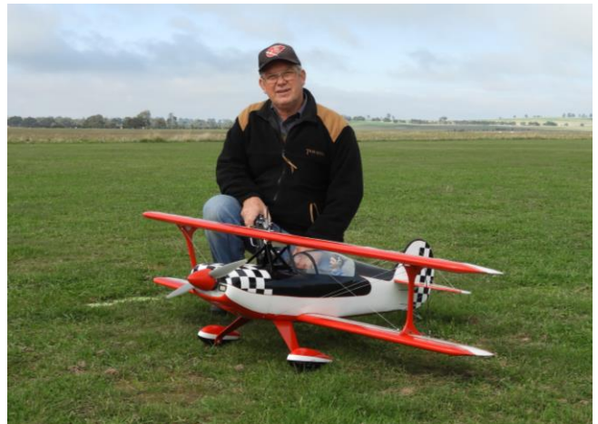
Peter Weston with his recovered Super Skybolt on Sunday 21 st May. It's covered with BEMS silk, dope and spray painted.
