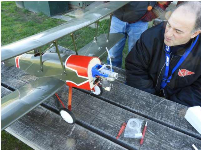
Back on the bench trying to sort out the crossed over fuel lines with Nick lending a hand. It is good practice to clearly mark the lines when you fit them to the tank (Carby, pressure/vent, drain etc.)
