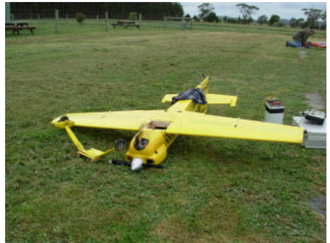
Glenn's CAP is back in the pits for examination of fuselage damage where U/C was torn out. Also sustained some minor damage to the wing.
