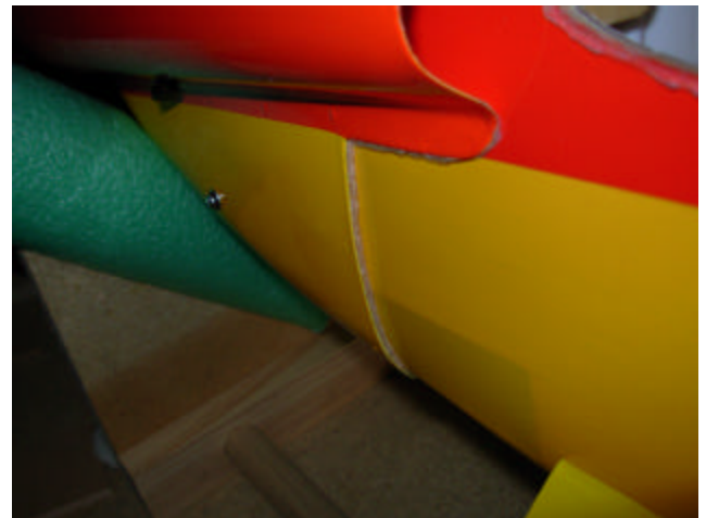
Electrical appliance packaging foam used to prevent fiberglass cowl chaffing the fuselage.
