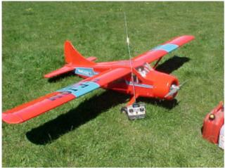
Sunday 9<sup>th</sup> November Graham Waterhouse brought out his new ARF Dornier DO-27 V.M.A.R Kit A.R.F 67 3/4" (1720mm) span 50" (1270mm) Long Engine - MDS – 46 Pitts Style muffler. Graham test flew the model during the week and is very pleased with its handling capabilities. He has made a few modifications to bring it up to his standard. Model looks very scale in flight and should do well in the up and coming scale competition.
