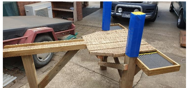
After picking up the cable from Hewitt & Whitty I found a length of 1" dowel in the garage and cut out two big washers from MDF scrap thinking we'd be hanging onto it while rolling out. Al suggested tying it to the trolley which worked a treat. Al is bending the wire to attach the pulley.
