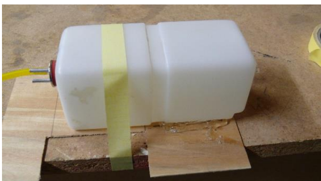
Whilst the below is not a very good photo, it shows the fuel tank with some silastic along the edge of the tank, there is plenty underneath.
