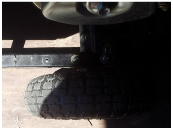
Axle moved back 55mm to stop it tipping over when wheeling forward. (Not a very good photo. It was taken after the generator was put back in the container and the sun shining in caused a shadow.)
