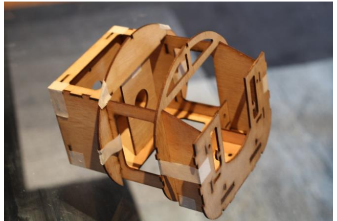
This photo shows all the parts assembled using the interlocking nature of the design and a bit of tape to hold it together.
