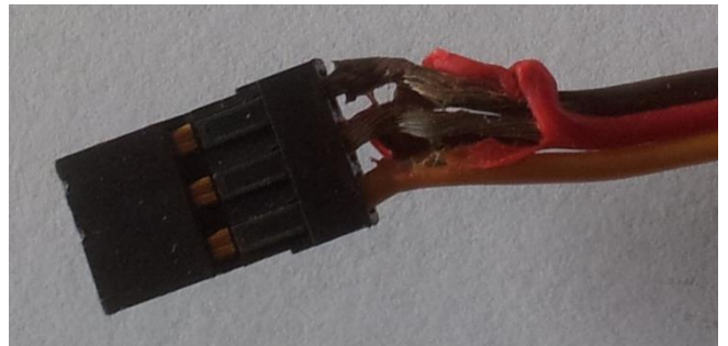
Throttle servo lead melted through the insulation.
