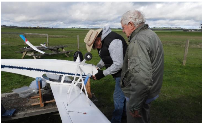
Graeme is doing an adjustment to the muffer and also the throttle linkage. As mentioned elsewhere, Glenn is having eye problems and finds close work difficult which is why he has asked us to closely go over the model.
