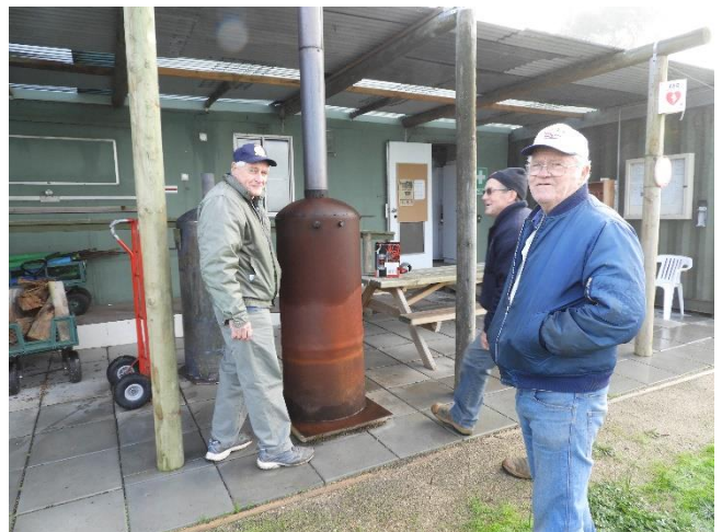
The old heater was full of holes up on top and was bellying out about 400mm up from the base. The cylinder wall was very thin at this stage after 4+ years of service.
