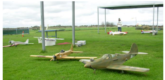
Norm Morrish's 1972 Northerner aerobatic model and my 1976 P39 Airacobra. Apart from age, both models have Kraft Multicon electric retractable undercarriage. The Northerner is powered by a Webra 61 2 stroke which is the same engine that originally powered my P39.
